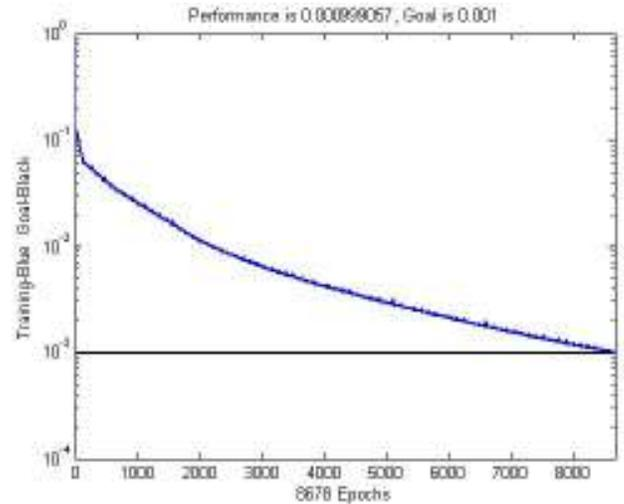
Figure 2. Cumulative Error versus Epoch plot for the FFNN
